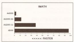
Figures 1-3: AIB benchmarks (in seconds) for the 3 machines. A1200 (1) were carried out with standard 68000 code, A1200 (2) with optimised 68020 code
