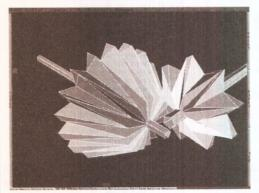
This is an example of one bevel gear driving another, at an angle of 90 degrees. This is probably the most common way of transferring drive from a given direction to another
