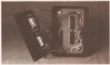
The circuit for the mouse-joystick switcher is really very simple, with all the components fitting on to a tiny piece of stripboard
