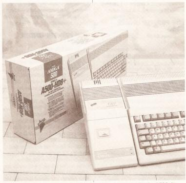
GVP's HD8+ is one of the fastest SCSI hard drives around for the A500. Its DMA-based design means it can bypass your Amiga's central processor and thereby ramp up throughput. It also looks pretty neat too..
