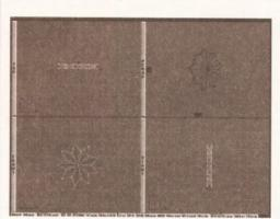
Once the inner points have been selected, they may be scaled down over the X and Z axis to create the teeth of the cog
