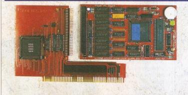
The KCS emulator is available as a trapdoor expansion for the A500 and A500 Plus, or with a plug-in card for the A1500/A2000/A3000 series. It comes with 1Mb of extra memory, too
